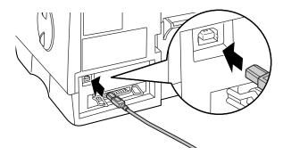
Insert the other end of the cable into the interface connector of your computer, or the USB hub connected to your computer.
